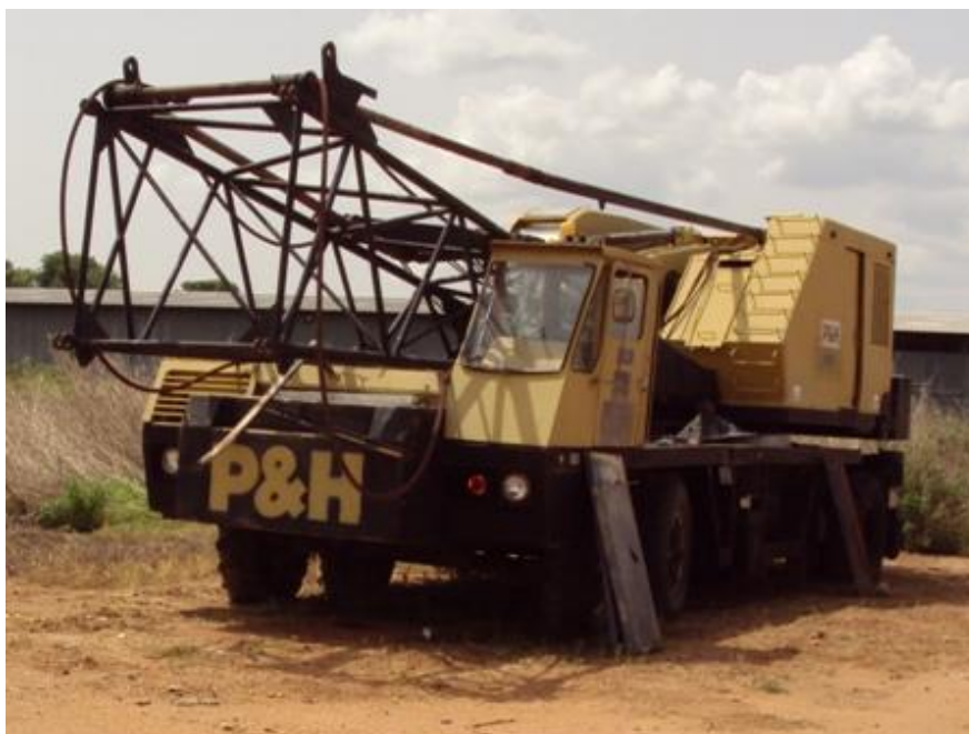
Photo 9.9: 30T Mobile Crane
