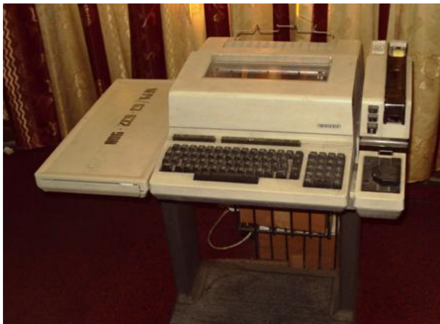
Photo 4.16: Old Siemens Sequence of Event Recorder
